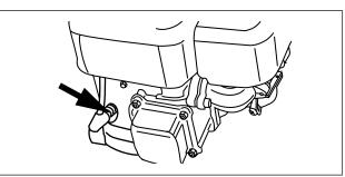
Figure 25. Typical Spark Plug Connection
